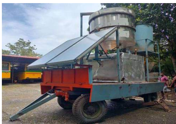
Trolley mounted essential oil distillation unit design and prototype
