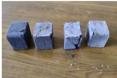
Bio-Cement Cubes after Failure in UTM
