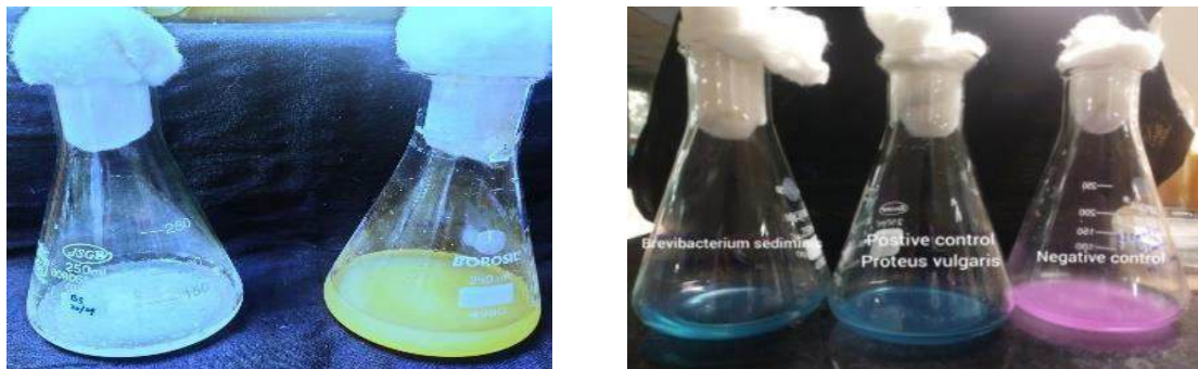
Fig. a. \text{CaCO}_3 Precipitation by Brevibacterium sediminis the left flask b. Calcium Carbonate Precipitation Test
